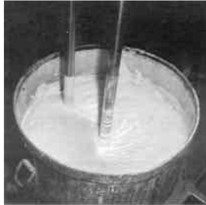
Stretch marks show the dispersing action of a Dual Range Disperser
