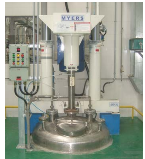
Model 600/800 Tank Mount Control panel is shown mounted close to the mixing machine. The drive is mounted away in a safe environment.
